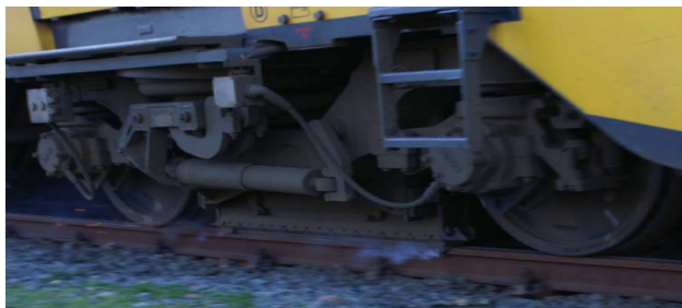
Figure 7.20 Magnetic track brake in action.
