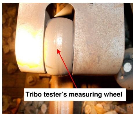
Figure 8.3 The tribo tester's measuring wheel developed by University of Twente.
