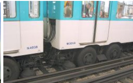
Figure 2.12 Subway train in Paris equipped with rubber tyres.
