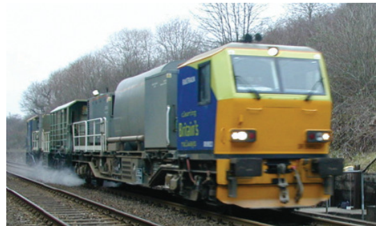
Figure 2.16 Water jetting; cleaning the track (England).
